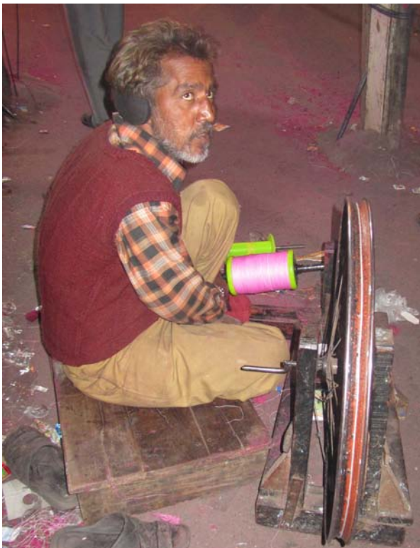
Coating of kite strings with glass
