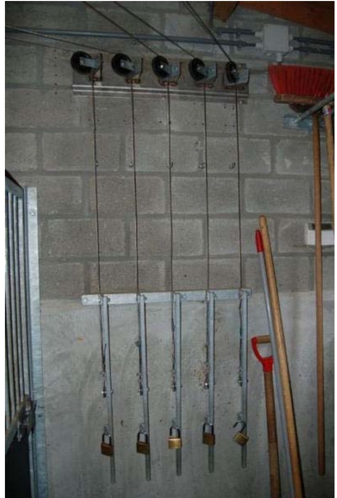
Fig 28. Levers - These levers make it easier for the keepers to move the sliding doors of the capybara enclosure. ©R.J. van Sluis, 2007
