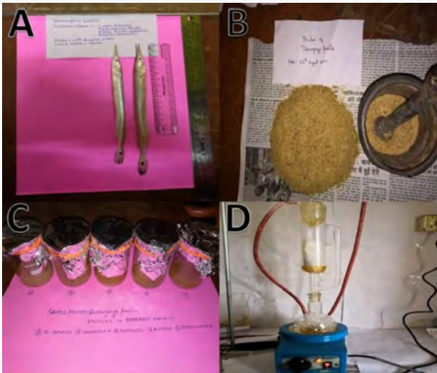
Experimental works on food of Indian Skimmer: A— D. pussila | B—Powder of fish sample | C—Extracts | D—Extraction.
